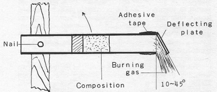
Figure 13. A whistling revolver around an axis by thrust inclination.
