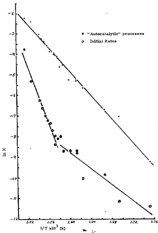
The Arrhenius plot for the TATB data is shown in the figure. The slope of the "autocatalytic process" gives an activation energy ( $E$ ) of 59.1 kcal/mole and the intercept gives a  $Z$  of  $3.75 \times 10^{18} \text{ s}^{-1}$ .
