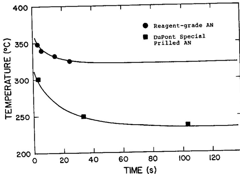
All of the tests in the figure were run on 0.8-mm-thick samples. A thicker sample gives a lower critical temperature. Results are quite sensitive to thickness, as would be expected from the  $a^2$  term in the Frank-Kamenetskii equation. Some care in sample preparation is rewarded with better precision in the results.
