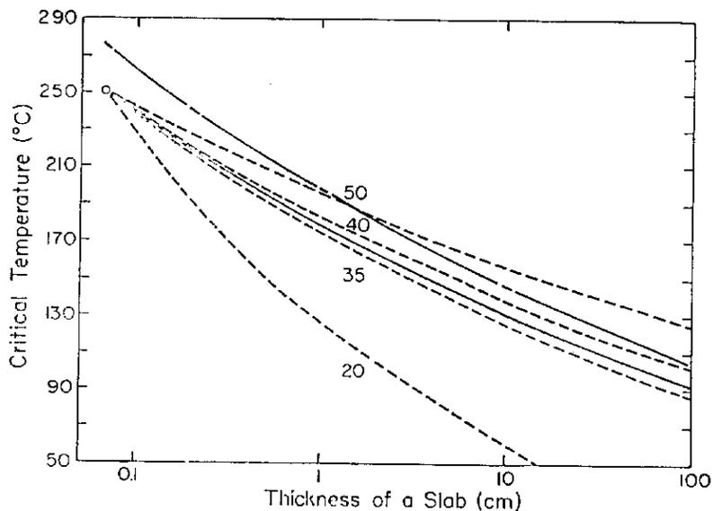
(benzenetrifuroxan) that has an experimental critical temperature of 250° C as a 0.6-mm-thick slab. An infinite number of compensating pairs of Es and Zs will predict the experimental  $T_c$ , but only the *correct* set will predict the critical temperature for all sizes and shapes.
