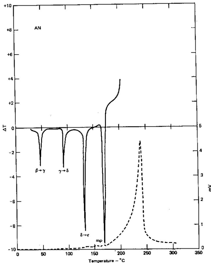
The downward peaks with negative  $\Delta T$ s indicate energy-absorbing processes. In the case of ammonium nitrate, there are three different changes in crystalline structure and melting. The melted ammonium nitrate starts to decompose exothermally immediately, and the curve rises into the  $+\Delta T$  range. The pyrolysis curve shows concomitant gas evolution.
