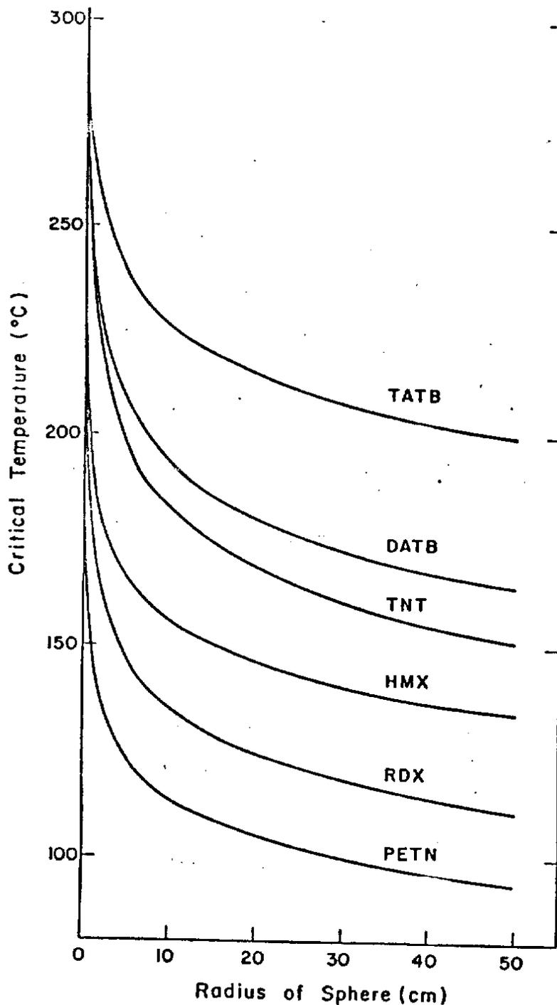
**The temperature at which any specific energetic material will self heat to ignition or explosion depends on its chemical properties, its size, and its shape.** The curves show that there is a specific critical temperature for each explosive at each specific size of sphere.
