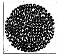
FIGURE 81. Ball Grains (Smokeless Powder) (3×). (Courtesy Western Cartridge Company.)
