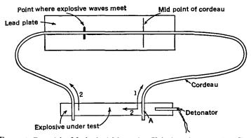
FIGURE 9. Dautriche Method of Measuring Velocity of Detonation. From the point A the explosion proceeds in two directions: (1) along the cordeau (of known velocity of detonation), and (2) through the cartridge of explosive which is being tested and then along the cordeau. When the two waves in the cordeau meet, they make a mark in the lead plate upon which the cordeau is resting.
