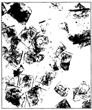
FIGURE 103 Diazodinitrophenol Crystals ( $90 \times$ ).
