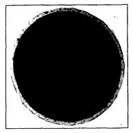
FIGURE 82. Cross Section of Ball Grain, Double Base, Deterrent Coated (112×). (Courtesy Western Cartridge Company.)
