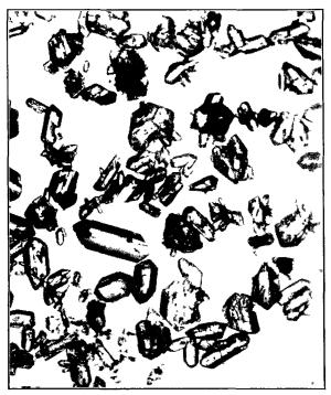
FIGURE 102. Lead Styphnate Crystals ( $90 \times$ ).
