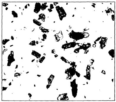
FIGURE 47. Commercial Sample of Purified TNT (25×).
