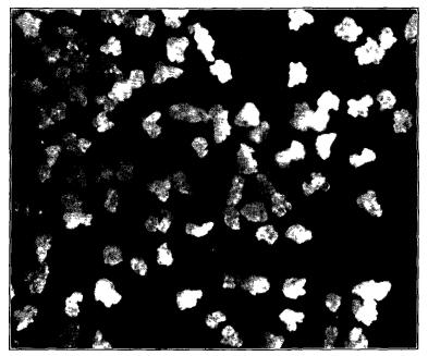
FIGURE 100. Technical Lead Azide, 90-95% pure  $(75\times)$ . For use in detonators. Precipitated in the presence of dextrin, it shows no crystal faces under the microscope.
